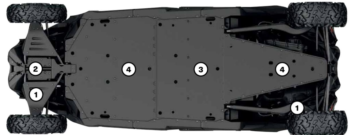
Our Plastic Plates glide smoothly and silently over obstacles, offering great protection in rough terrain. Made of abrasion-resistant thermoformed 3/8" (10 mm) thick High Molecular Weight Polyethylene (HMWPE).
